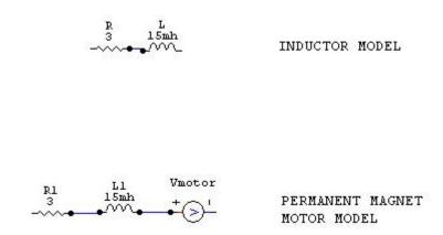
As can be seen from the models the permanent magnet generator is modeled with a voltage source. The voltage source is normally proportional to the speed. The voltage source adds a very important aspect with large implications.
