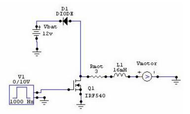
Most of the principles of DC-DC converters apply to chopping technique. The main differences are the variable motor voltage and the motor inductance. In the design of a typical DC-DC the designer chooses the optimal inductance. Inductances in DC-DC converters are typically in the micro Henry range not the tens or hundreds of milli Henry range for motors. The switching frequency will then need to be lower and possibly variable to match the motor inductance.
